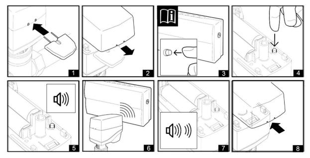
The buttons and LED displays that are used during commissioning are located inside the housing. Remove the housing cover before commissioning (1/2).
