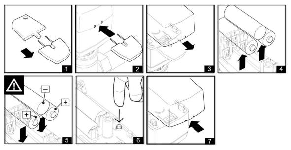
Open the battery lid using the key supplied (1) by inserting both pins into the intended place (2). Remove the cover (3).
