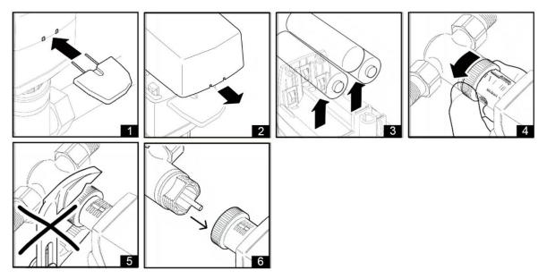
Open the battery compartment cover using the key supplied (1) by inserting it into the intended place. Remove the cover (2). Remove the batteries (3). Loosen the union nut (4/5). Remove the SAB05 from the valve (6).
