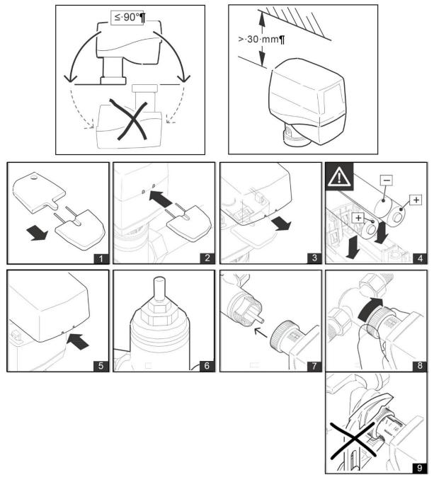
Open the battery compartment cover using the key supplied (1) by inserting both pins into the intended place (2). Remove the cover (3). Insert the batteries correctly (4) and close the battery compartment cover (5). Place the SAB05 onto the threaded connection of the valve (6/7) and tighten hand-tight using the union nut (8/9).
