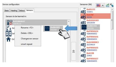
Sensors and devices, within range, are listed on the right side of airConfig. To learn in a specific sensor simply drag and drop the (activated) symbol into the sensors input tab of the STC-DO. The Sensor's (EEP) type must be known to be assigned correctly through activation of the sensor or switch. The sensor type is coded in the EEP, which is included in the sensor's LRN telegram.
