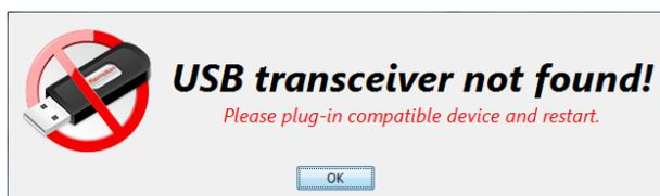
In this case please check in your WINDOWS Device manager whether the USB transceiver has been detected properly and the driver is installed. If the driver is missing, you may download the appropriate driver for your system from <http://www.ftdichip.com/Drivers/VCP.htm>
