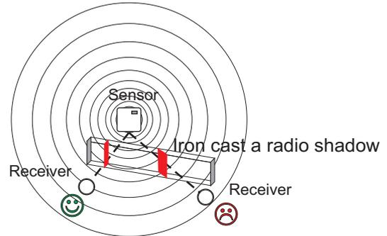
In addition, the angle with which the signal sent arrives at the wall is of great importance. Depending on the angle, the effective wall strength and thus the damping attenuation of the signal changes. If possible, the signals should run vertically through the walling. Walling recesses should be avoided.
